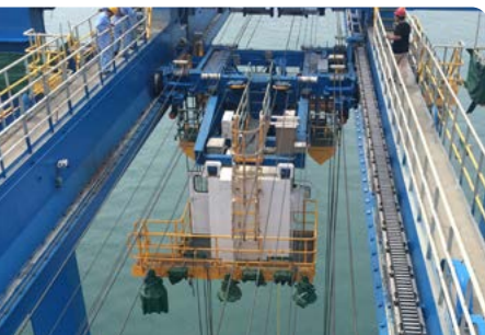
Ship to shore crane with roller supported chain system
