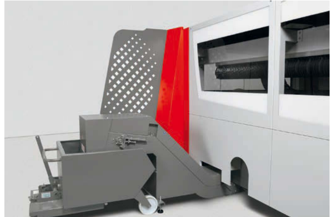
Teileaustrag über Querförderer in Container. Discharge of parts into the container by the cross conveyor.
